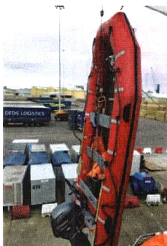
Rescue boat – hanging vertically because strops have not been fitted correctly
